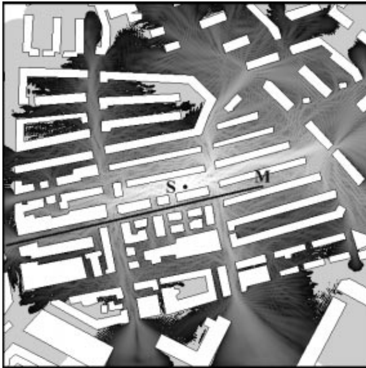
FIGURE 4.11: Layout and result of simulation for the complete urban microcell located in the center of the city of Bern; the simulation arrays are of size 600 \times 600 . “S” marks the source location and “M” the measurement axis. Gray scale is distributed between 30 dB (white) and 120 dB (black). The field intensity measurement is given in 4.12
